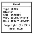
The About menu displays the type, class and serial number, version and HWID (hardware ID) of the sound level meter.
