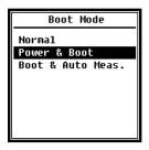
In Start mode, use the arrow keys  $< \blacktriangle >$ ,  $< \triangledown >$  to select Normal, **Power & Boot**, and **Boot & Auto Meas.** (Switch on and Auto Meas.).
