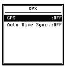
In the GPS menu you can enable or disable the GPS and Auto **Time Sync** options. When the **GPS** is disabled, the internal GPS module is turned off. The system clock of the sound level meter will synchronize with GPS time if you enable the Auto Time Sync option.
