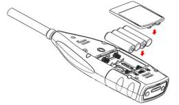
Replace the batteries and close and lock the battery compartment.
