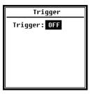
In the **Trigger** menu you can switch the function of the trigger on and off. The **trigger** is an analog input with which you can start or stop the measurement for the sound pressure meter by remote control. The trigger input is located on the bottom of the sound pressure meter (headphone jack 3.5 mm).
