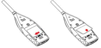
Turn the shutter to the left to remove the battery cover. Lift off the battery cover.
