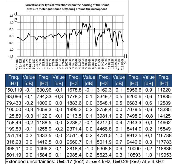
Note: The frequency marked with \* is not prescribed in the standard, the exact frequency can be found in IEC 61672-1.
