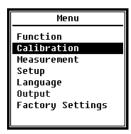
Press the <Menu> button **to** enter the next menu. All measurement parameters can be set in the menu.
