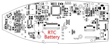
☆Note : The system clock of the sound level meter was calibrated with a reference clock with an average error of 2 ppm (maximum error 3 ppm). The time accuracy is less than 10 ppm at room temperature (<26 seconds within 30 days). The maximum time error for internal tests at 25 °C was about 5 to 8 seconds.
