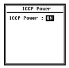
The ICCP menu controls the power supply of all ICCP sensors via the 24 V/4 mA constant current source. Disable the ICCP power supply before connecting another sensor or connecting directly to the signal source. Press the arrow keys < 4>, < >> to select.
