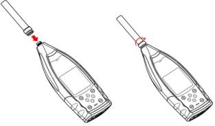
Connect the microphone to the TNC connector. Then turn the thread until the parts are firmly connected.
