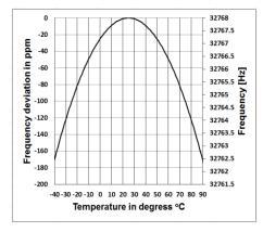
The accuracy of the system clock may vary depending on the temperature, as there is no temperature compensation. With the typical temperature curve in the illustration, the system clock does not change its base frequency. If the temperature rises or falls, the frequency of the system clock changes by about -0.04 ppm/° C<sup>2</sup>. Therefore, if the temperature is 0 ° C, the value for the system clock changes by -0.04 x (0-25)<sup>2</sup> = -25
