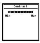
**The Contrast** menu allows you to adjust the contrast of the LCD display in 14 levels. Press the arrow keys  $< \blacktriangle >$ ,  $< \lor >$  to select.
