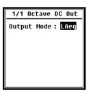
**1/1 Octave DC Out** defines the output signal in 1/1 octave mode. The following options are available: LAeq, LBeq, LCeq, LZeq, 31.5 Hz, 63 Hz, 125 Hz, 250 Hz, 500 Hz, 1 kHz, 2 kHz, 4 kHz, 8 kHz, 16 kHz. Press the arrow keys < 4>, < > > to select.
