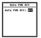
The sound level meter has an automatic switch-off function to reduce power consumption. If the sound level meter remains in stop status and no button is pressed for a certain period of time, the instrument will shut down according to this setting. The following settings are available for the auto power off option: **1 minute**, **5** minutes, **10 minutes**, **30 minutes**, **Off**. Press the arrow keys < **>**
