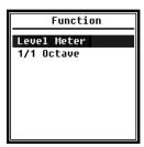
Select the **function** and press the < Enter> button to enter this menu. You can select 2 measurement types: **Level measurement** and **1/1 octave measurement**. Press the arrow keys< $\blacktriangle$ >, < $\Psi$ > to select the measurement mode. Press the <Enter> button to save the setting and return to the previous menu. Press the <ESC> button to return to the previous menu.
