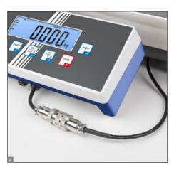
■ Verification plug, for verified balances this enables you to separate the display device and platform without affecting the verification, e.g. for installing the scale in a packing and dispatch table, pit frame etc. at a later date.
