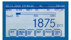
Professional counting function All relevant counting information at a glance, such as, e.g., reference weight, reference quantity, total count, total weight, tare container weight, available weighing capacity and much more
