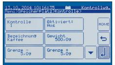
80 memories for each mode e.g. for Checkweighing, PRE-TARE, reference weight, target value when dispensing, item descriptions, user name, weights for tare containers, etc. Easy to enter using the large-scale keypad
