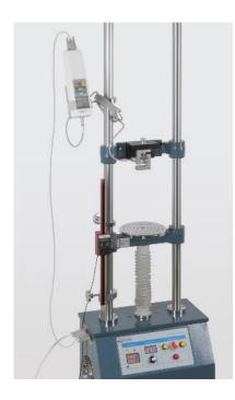
• The force gauge screwed to the test stand is now connected to the test stand at the equipment port by means of the RS232 cable
