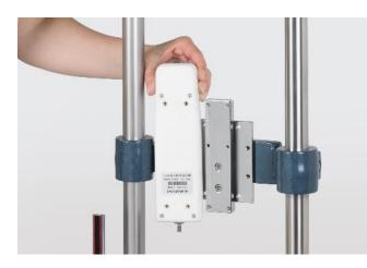
• Force gauges with internal sensor by means of the adapter plates to the crosshead (4x M3x8 cylinder screws).
